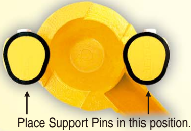
Figure 1. Settings for Ladders 65mm - 78mm.
